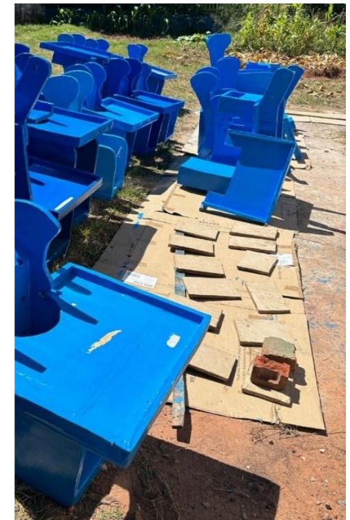
APTERS workers glue three pieces of cardboard together to create a sturdy material which is then cut into a physiotherapist-designed frame. The frames are coated with oil-based paint to make them water resistant, and cushions are sewn for added comfort.
